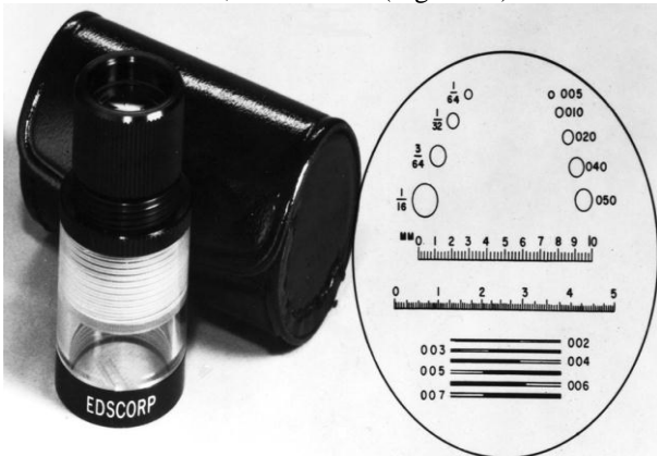
Fig. 3.1.1—Comparator for measuring crack thicknesses
